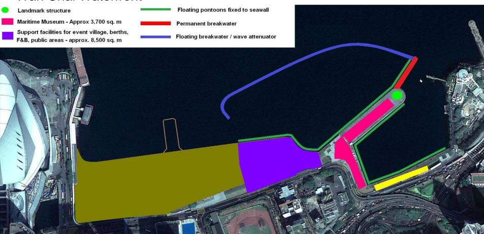
Wan Chai Waterfront Park – Integrated with the Ex-PCWA and incorporating a floating breakwater / wave attenuator, pontoons for large visiting yachts, public landing steps and shaded promenade, waterfront performance area, public space / park that is so designed to enable temporary overlay of an event village provisioned with appropriate infrastructure and access
