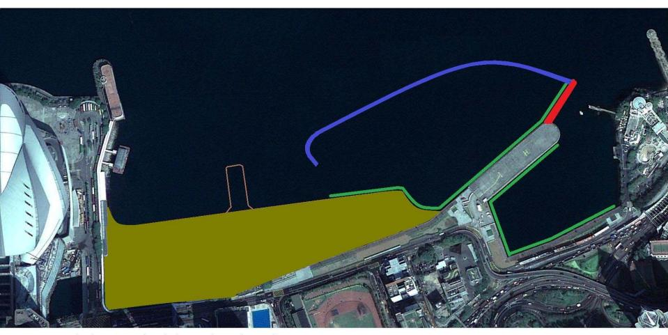
Permanent breakwater - required to make the existing basin Typhoon proof
