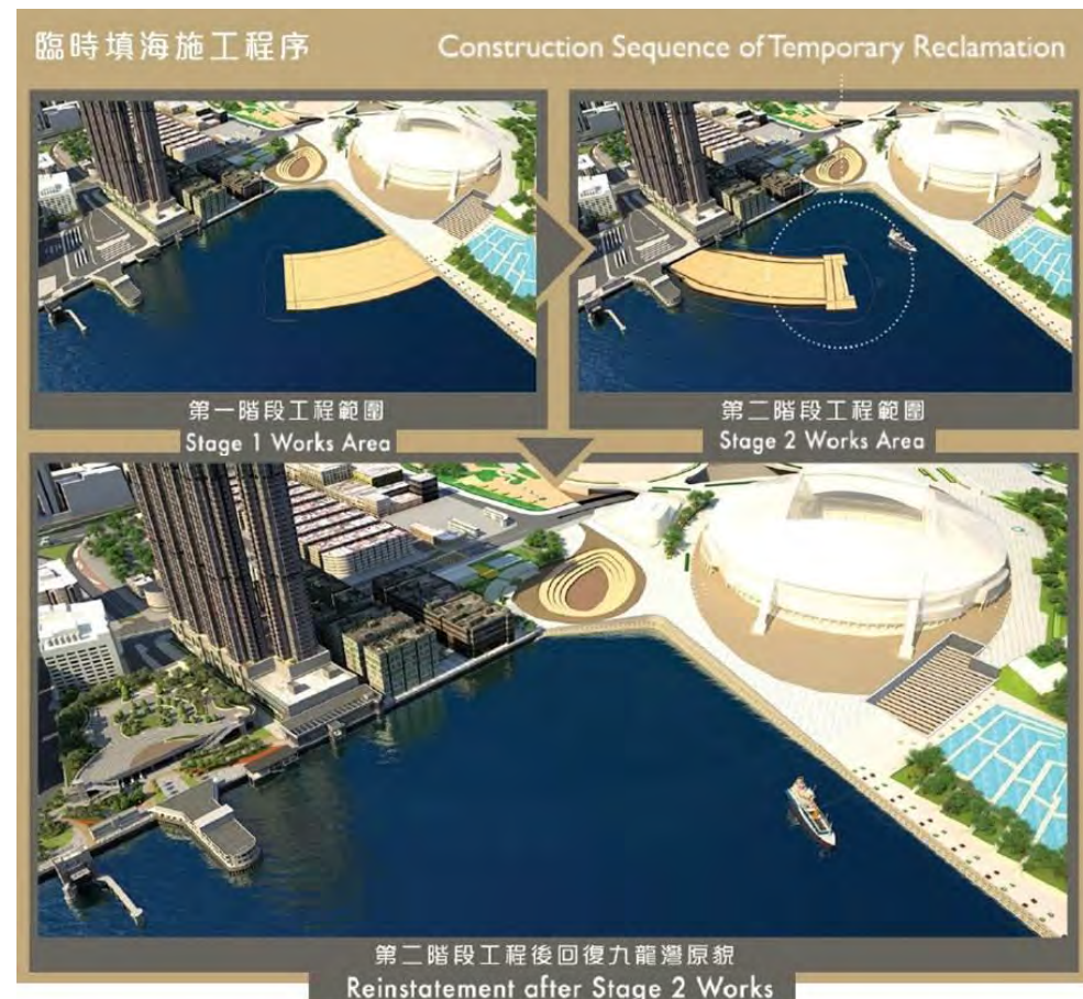
Figure 3-16 – Two Stage Temporary Reclamation Arrangement in Kowloon Bay
