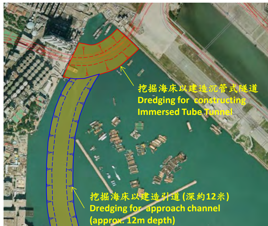
Figure 3-6 – Dredged Trench and Approach Channel for IMT
