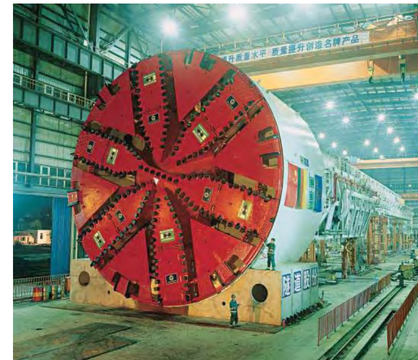
Fig. 4 Tunnel Boring Machine (about 14m Diameter)
