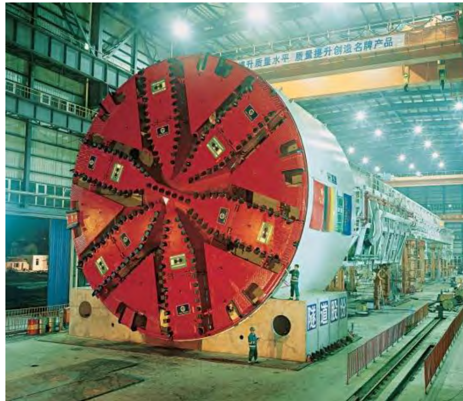
Figure 3-8 – Tunnel Boring Machine (TBM)
