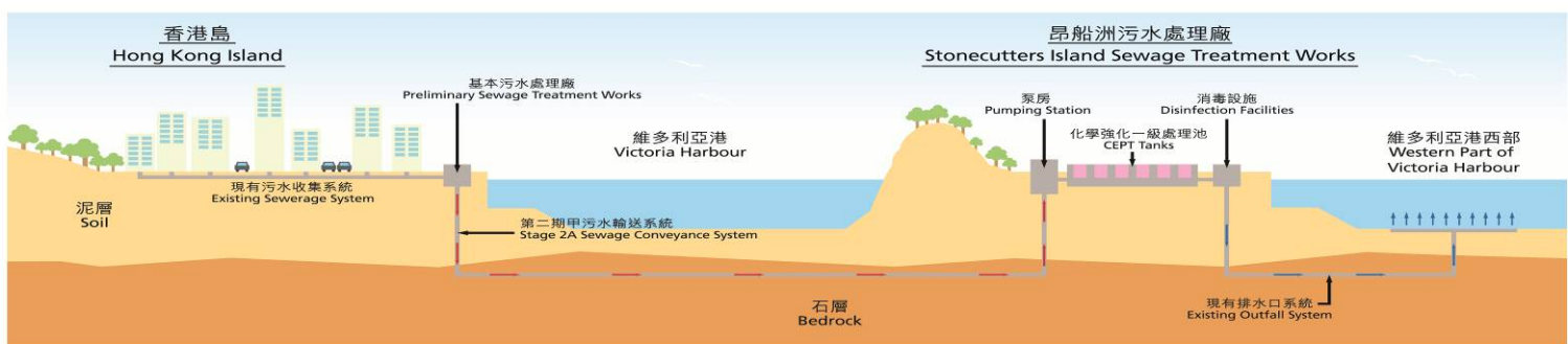
Figure 5 – Sewage treatment under HATS 2A
