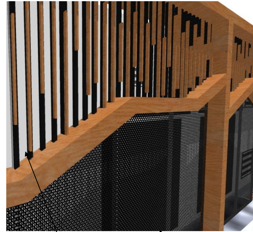
PERFORATED METAL PANEL STRUCTURAL FRAME AND VERTICAL FINNS: ALUMINUM-RECYCLED WOOD PLASTIC COMPOSITE
