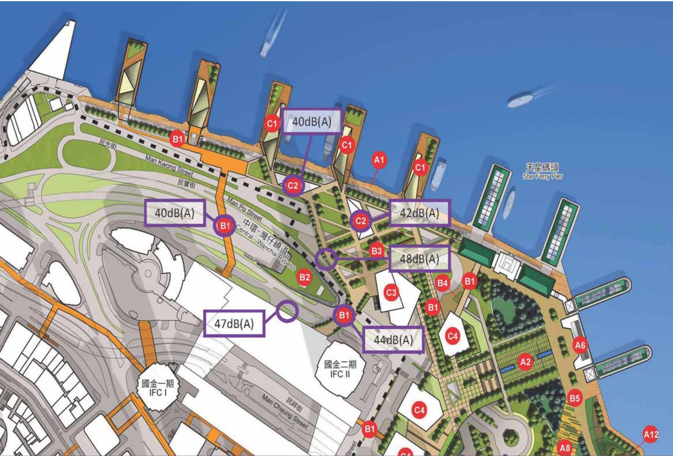
Annex 4 NOISE LEVELS IN THE VICINITY OF WVB AT ITS OPERATION MODE
