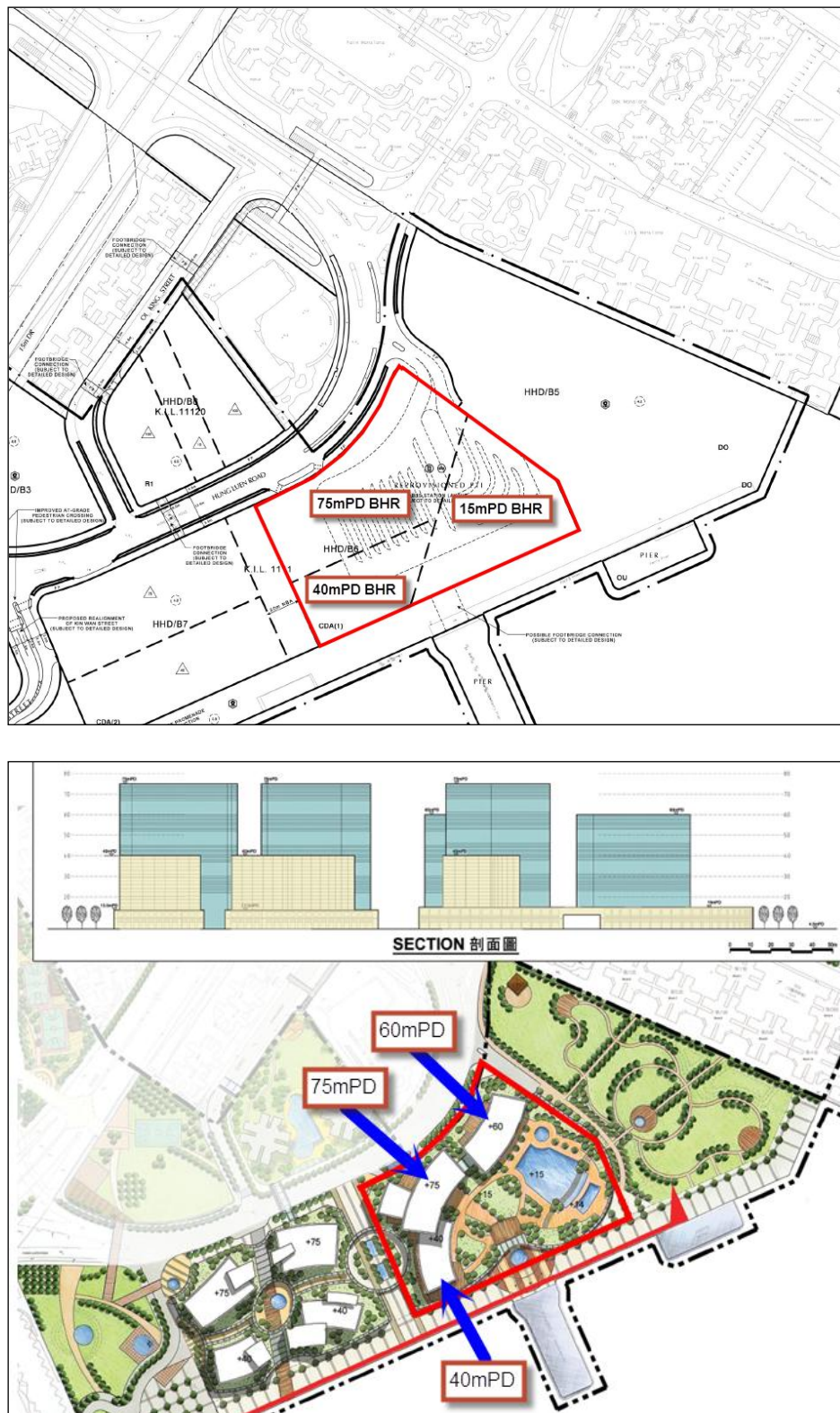
Figure 3.1 – BHRs and Indicative Built Form of the Site Proposed in the Hung Hom District Study
